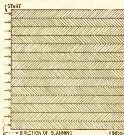
Fig. 3-a—The usual horizontal scanning path.
